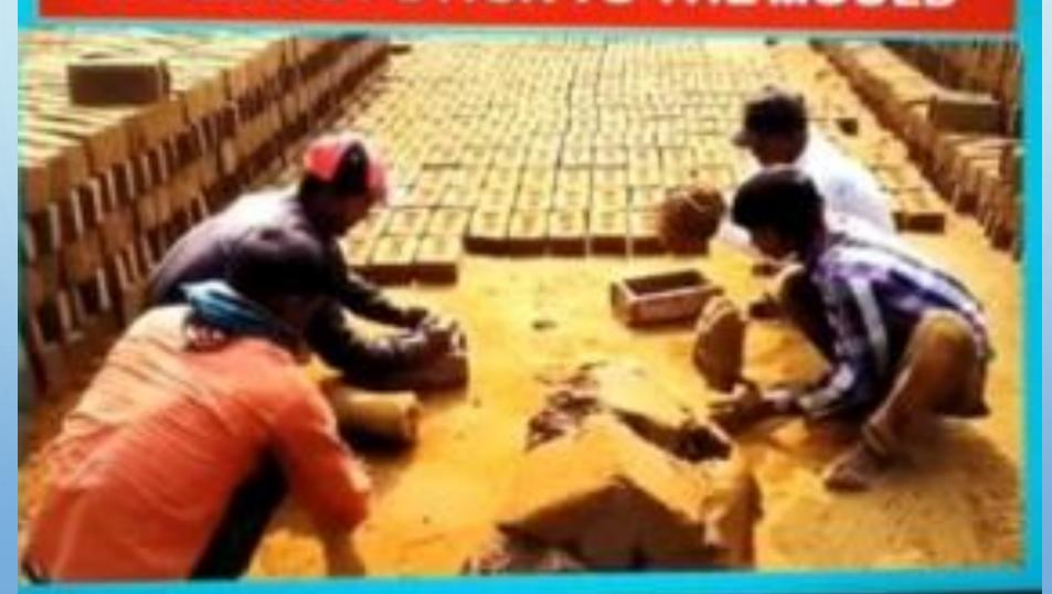
THE MOULD IS EMPTIED ONTO THE DRYING AREA. AFTER EVERY TWO DAYS THE BRICKS ARE TURNED OVER FOR UNIFORM DRYING. THEN THEY ARE READY FOR BAKING.
